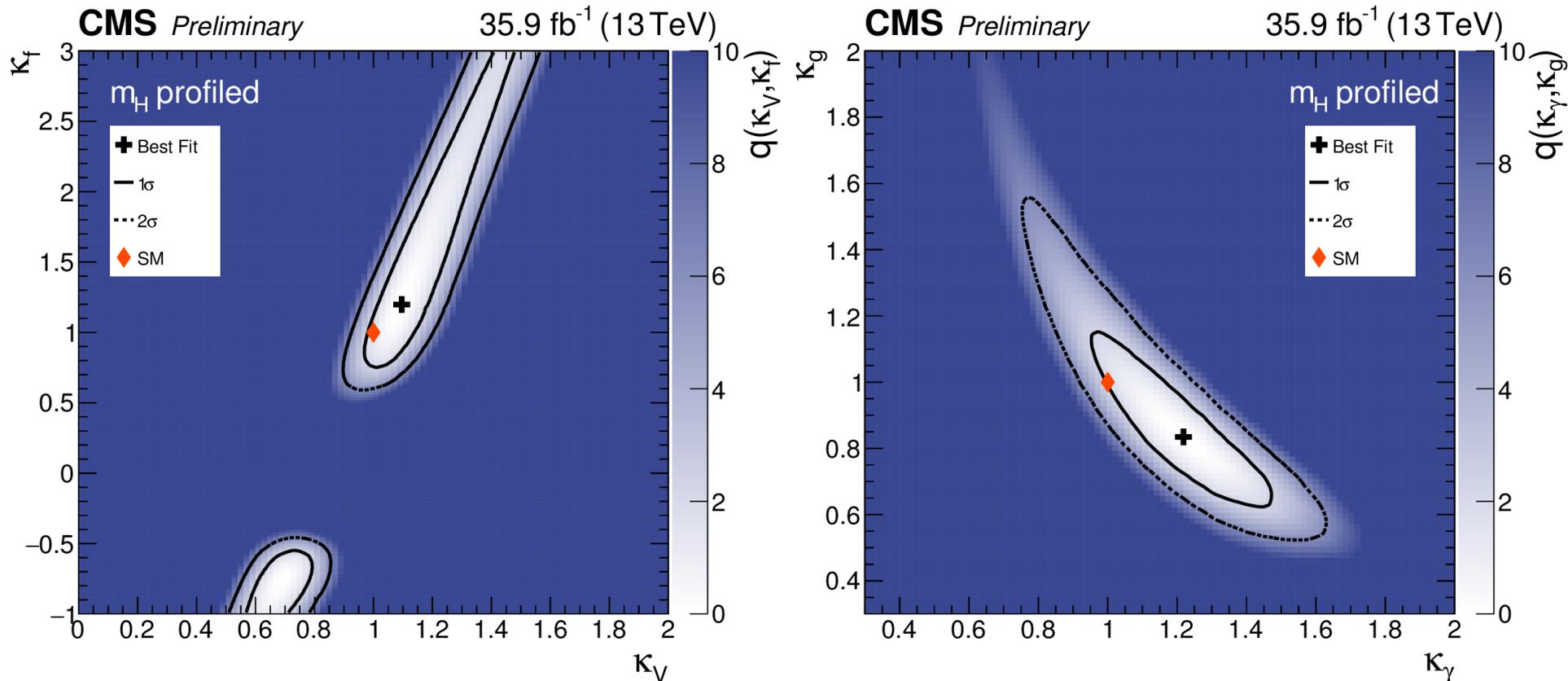
Two-dimensional likelihood scans of  $\kappa_f$  versus  $\kappa_V$  (left) and  $\kappa_g$  versus  $\kappa_\gamma$  (right) based on the H $\rightarrow\gamma\gamma$  decay channel. All four variables are expressed relative to the SM expectations. The mass of the Higgs boson is profiled in the fits. The crosses indicate the best-fit values, the diamonds indicate the Standard Model expectations. The color maps indicate the value of the test statistic  $q$  as described in CMS-PAS-HIG-16-040.
