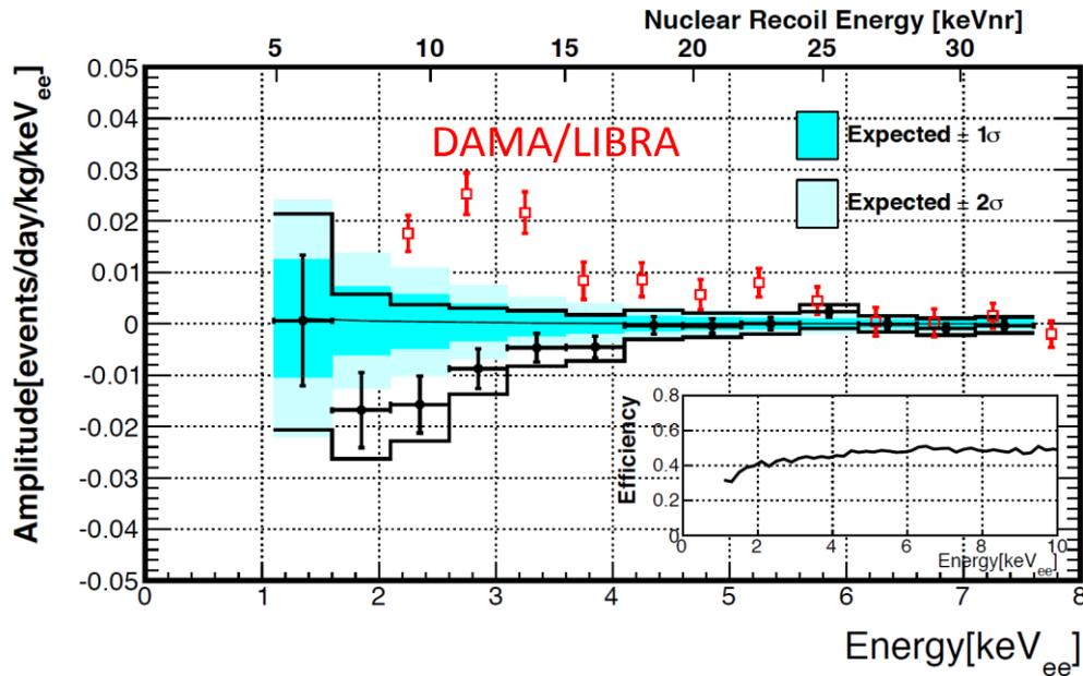
Annual modulation signal is searched for without any model assumption. Phase and term are fixed at  $t_0=152.5$ days and  $T=365.25$ days, respectively. following equation.
