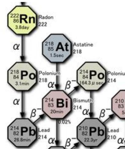
Remaining events can be explained by background events produced by radon in liquid xenon. By  $^{214}\text{Bi}$ - $^{214}\text{Po}$  coincident analysis, radon concentration is estimated to be  $8.2 \pm 0.5 \text{ mBq/detector}$ . Based on this estimate, most right column shows the # of expected background events from  $^{214}\text{Pb}$ .
