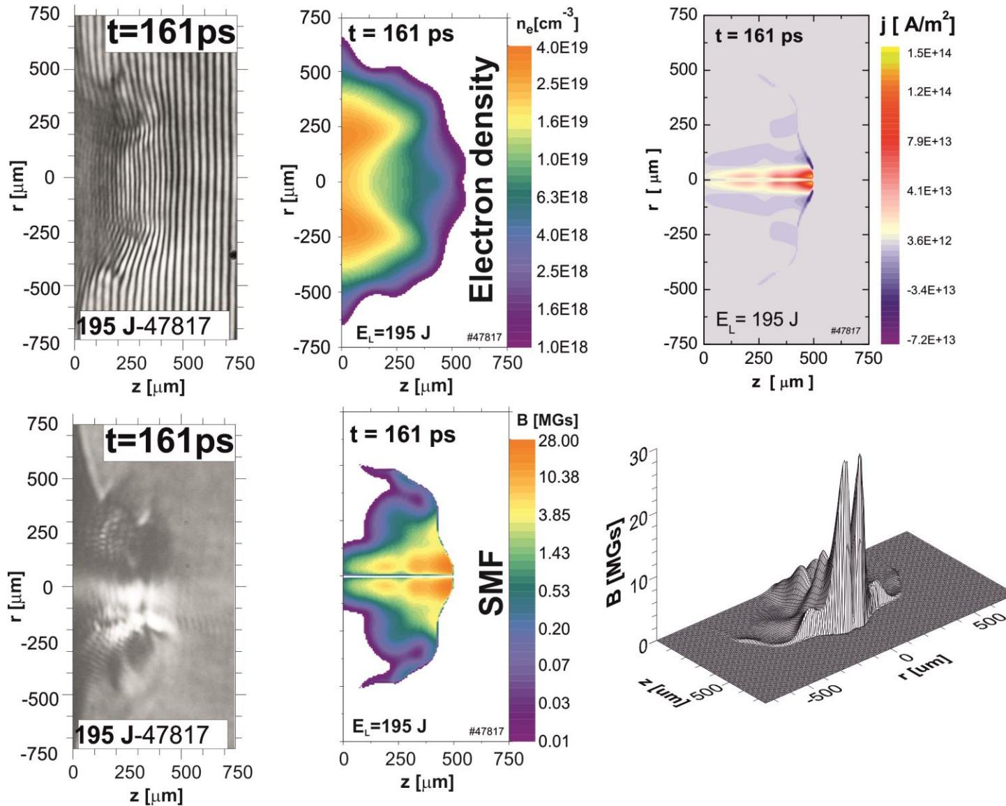
Space-time distributions of the SMF obtained during the laser pulse interaction with targets (made from different materials) fully demonstrated usefulness of this diagnostic system for investigations of SMF in laser-produced plasmas
