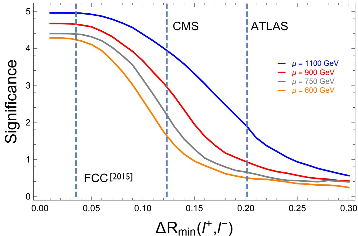
DELPHES FCC card used has 0.035 resolution in  $\Delta R$  ( $\eta=0.025, \varphi=\pi/128$ ).
